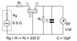
Including stray capacitance and input capacitance of RF voltmeter
